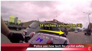
Chattanooga, Tennessee police have been testing a tool attached to the bike handlebars that indicates if a car driver has passed the bicycle closer than 3 feet. The bicycle police officer can catch up with the driver at the next light and give them a warning and information about the safe distance for passing bicyclists.
