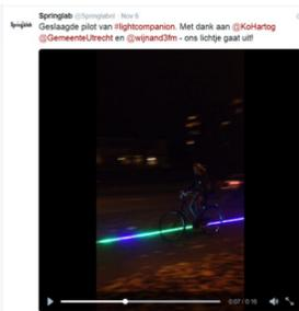
will arrive at the intersection and have a green light. This allows for the bicyclists to keep up their momentum. The green wave has also been tested in an LED tube that parallels the cycle track. If the bicyclist can pedal at the speed of the green light within the tube, they will arrive at a green light. These parallel-to-the cycle track light tubes also show the outline of the cycle track at night. If there is snow, the green wave small posts would better inform the bicyclist than a tube
