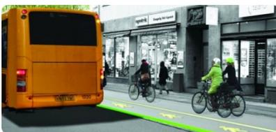
In Copenhagen, bus stops are preferred that offer a full island for waiting bus passengers but often the street is not sufficiently wide. Lights in a line that parallels the cycle track will be green when there is no bus at the bus stop but lights will be activated across the full cycle track when bus passengers have priority.
