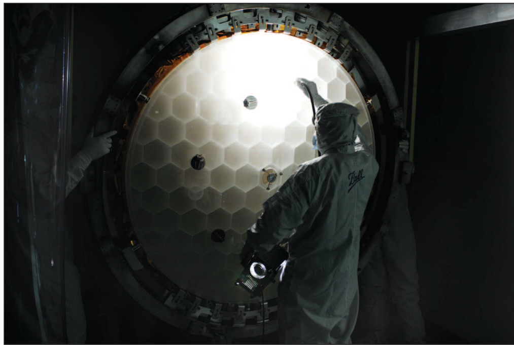
NASA and Ball Aerospace The honeycomb structure of Kepler's primary mirror makes for an extremely light weight — only 14 percent of a solid mirror of the same dimensions.
